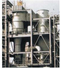
High Efficiency Cyclones. These are the most cost-effective solution for filtering particulate 5 microns or heavier. More than four decades of experience produce designs with low pressure drop and low operating costs.
