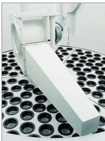
Integral Cleaning Fan and Manifold—The MikroPul Reverse Air bag cleaning operation is accomplished by effectively using a simple reverse flow fan. The fan and manifold rotate above the tube sheet and filter bags, eliminating friction and metal-to-metal contact. There are no valves, dampers or compressors to maintain. And with the absence of compressed air, there is less risk of explosion because no additional oxygen is being introduced.
