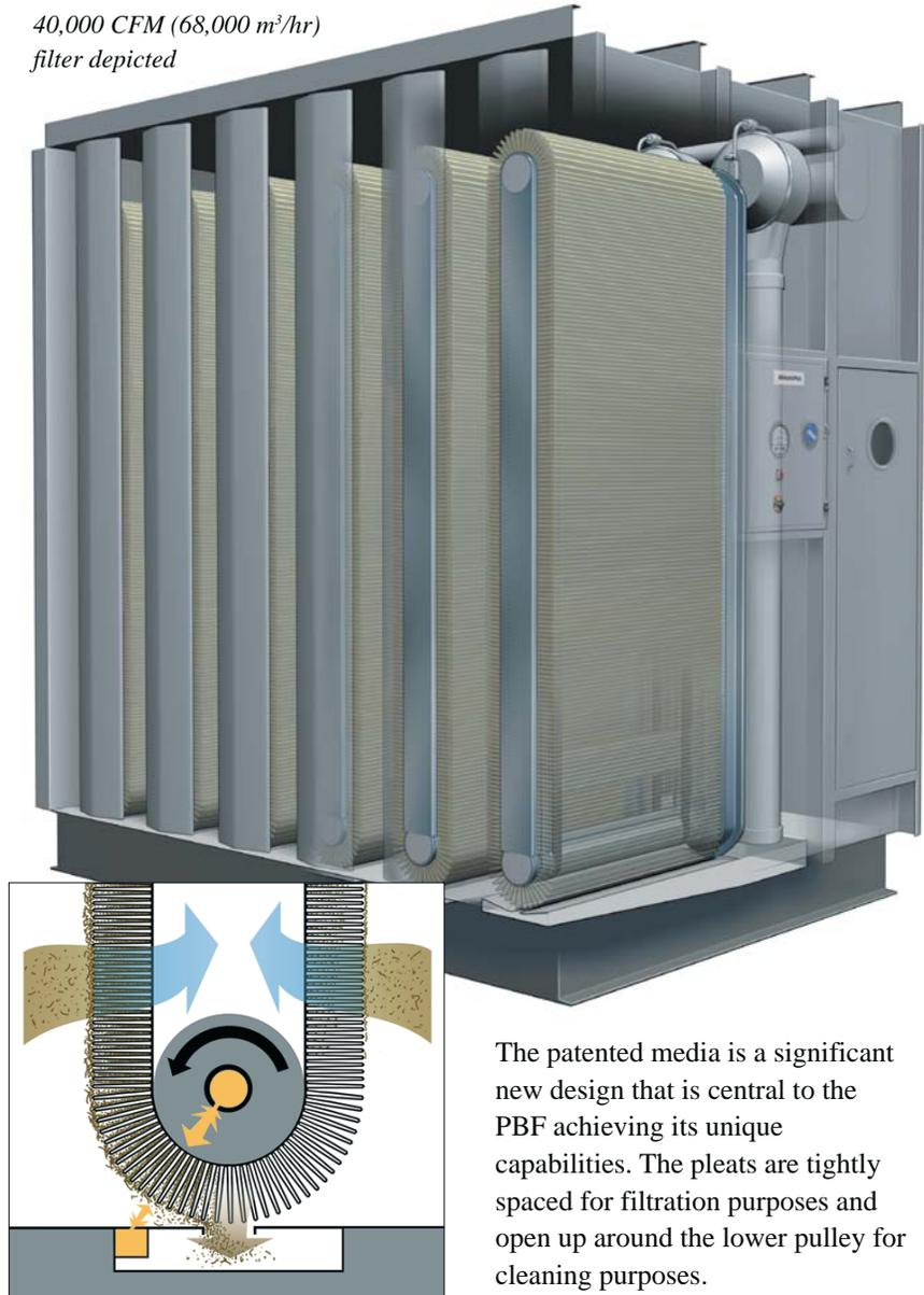
The patented media is a significant new design that is central to the PBF achieving its unique capabilities. The pleats are tightly spaced for filtration purposes and open up around the lower pulley for cleaning purposes.
